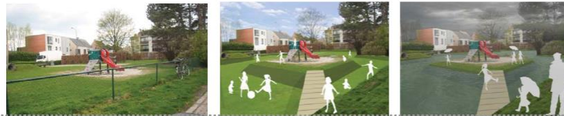
Proposal to convert an existing playground into a multi-use water infiltration/retention facility
